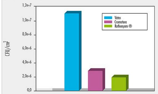
Resistance to bacterial growth on glass compared with that of chromium plated and ruthenyum ® plated surfaces. The bacterial colonies (CFU) grown after 72 hours on chromium and ruthenyum ® plated surfaces are respectively 74% and 82% less than those grown on glass surface.
